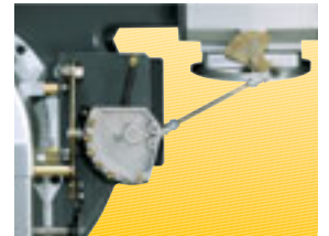
Example of the variable profile cam on RS 70-100-130 burners.
